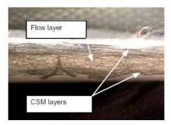
Ahlstrom Combiflow is a special reinforcement for closed mold processes.
